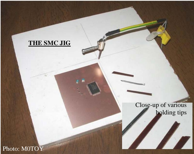
The Frame is simply twin stiff wire, anchored to the R/H edge of the board, and ending up with a 2-screw connector sleeve—the lower one being an oversize screw which can easily be loosened or tightened to grip the holding tool (tip). A selection of these holding bits are shown by the PCB, cut to match a variety of SMCs. [There's even a small plastic pocket (yellow, r/h edge) to store these bits ! ]
