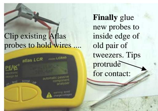
Clip existing Atlas probes to hold wires ....
