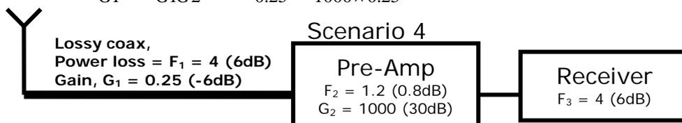
This is 6dB down on having the pre-amp at the antenna. So the case still stands, and that's why you always should have low noise pre amplifiers as close to the antenna as possible to improve the systems performance in response to noise.
