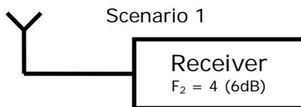
Lets start off with a system of antenna, coax and rig, NO pre-amp at the moment, look at **Scenario 1**. The rig connected directly to the antenna, I didn't choose the noise figure of 4 for any reason, just as an example. Clearly the noise figure of this system is  $F = 4 = 6\text{dB}$
