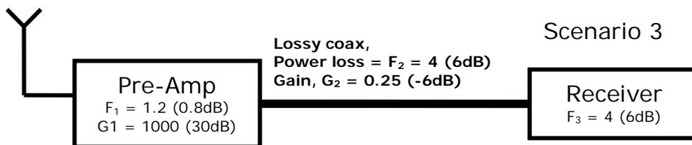
This is clearly a huge improvement, even better than having the aerial directly connected to the receiver, all on account of having low noise and high gain to counteract degradation later in the system. Now the ultimate test, what if you put the Pre-Amp directly into the receiver as in Scenario 4:
