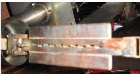
And finally, here's part of the 24 GHz GB3ZME microwave beacon which has been re-furbished ready for the 2011 portable season. 10 microwave slots are visible, with 10 more on the reverse side. A further 20 slots are not visible here. The dis-colouration was due to moisture ingress.
