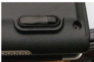
Third, my workhorse laptop, one of its feet had fallen off, and the power lead was intermittent. The power lead connector was dissected, lead trimmed and re-soldered, then the connector got the Sugru treatment.
