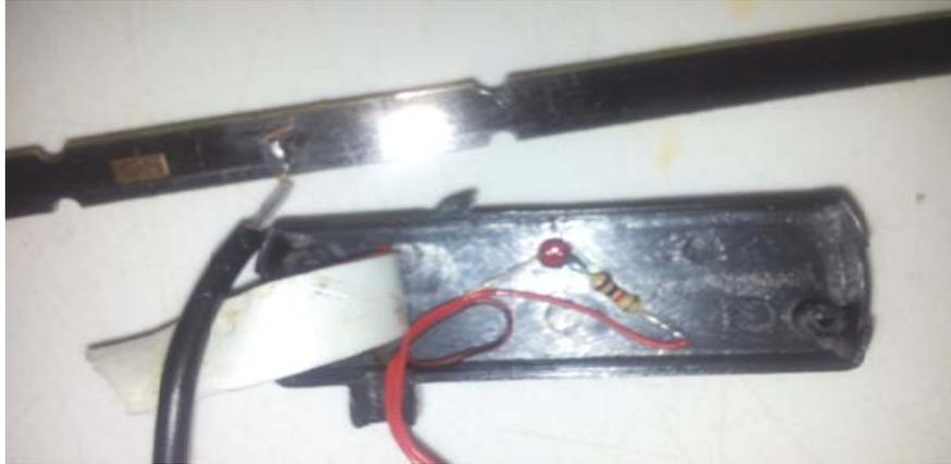
So I thought I would remove the amplifier lead and make the PCB aerial into something semi-decent.
